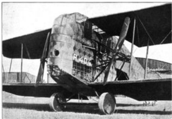
THE LINKE-HOFMANN R.1: View of the cabin and airscrew mounting.
